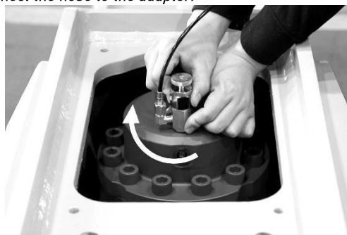
4. Conecte la manguera al adaptador. Connect the hose to the adapter.
